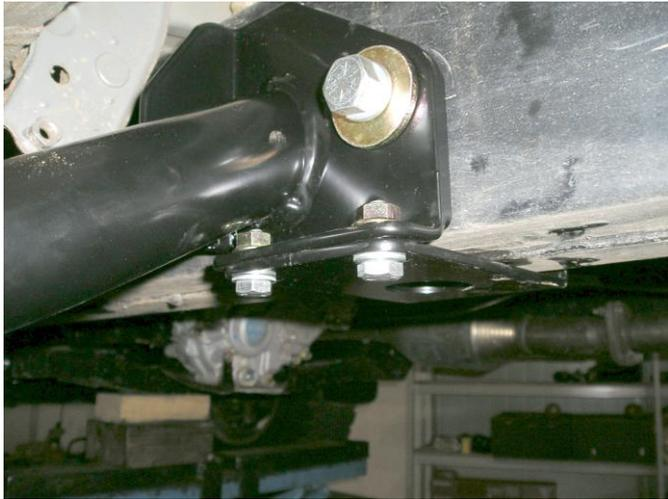
**11. Using two M8 x 20mm bolts, M8 flat washers and M8 flange nuts, secure the clamp to the centre support tube.**
