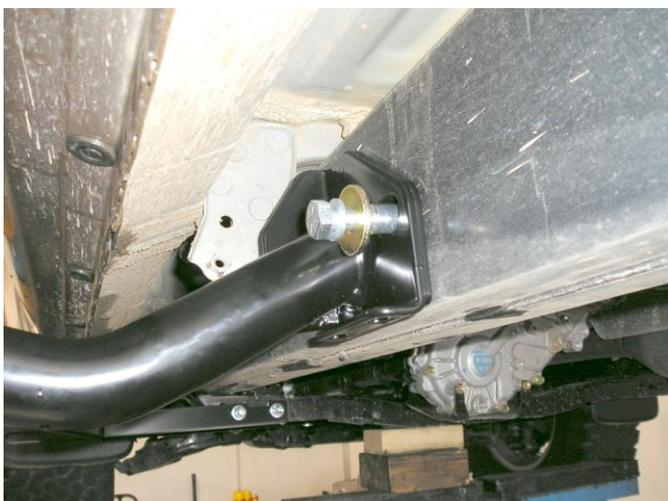
10. Using a 1/2" x 4 1/2" bolt, 1/2" spring and flat washer and a sleeve, join the centre mount to the clamp bracket.
