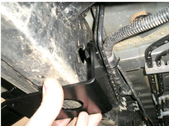
9. Attach the centre mount to the chassis by first placing the centre clamp bracket on the inside of the chassis. (note the welded on nut fits in the hole on the inside of the chassis)
