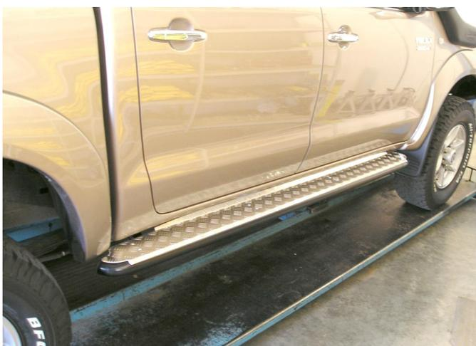
21. Run a bead of silicon along the length of the side step where the checker top will contact. This helps eliminate vibration.
