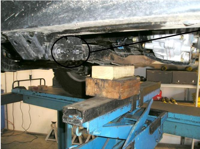
3. Working on one side at a time, support the gearbox cross member and remove the two outer bolts. Discard the bolts.
