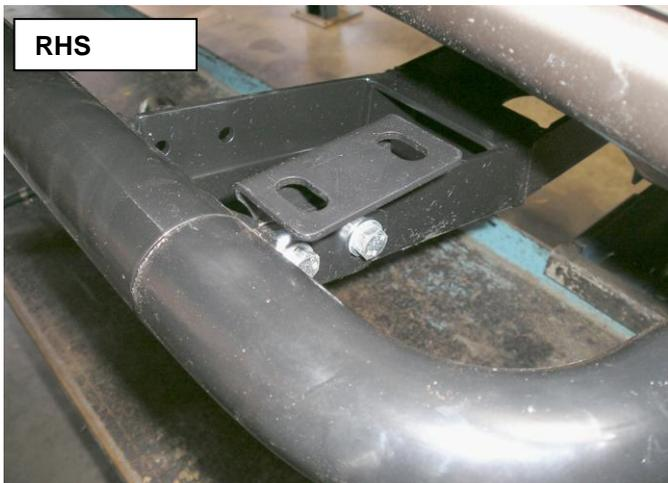
20. Align the end cap so that it sits level with the side step. Tighten the bolts joining the end cap to the step.
