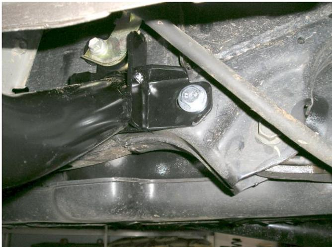
7. Loosely attach the rear mount to the chassis using a M10 x 35mm bolt inserted from the outside, a M10 flat washer and a M10 flange nut.
